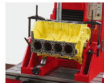
30° and 45° V-fixture (for boring)
